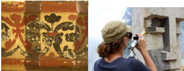
Figure 1. Laser cleaning on mural painting and stone
