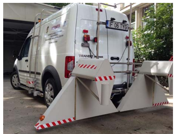
Figure 4. Equipment for the road longitudinal and transversal profile testing
